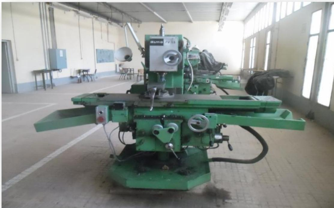
Figure II-17- Machine-outil (Fraiseuse ALMO FV1.5)
