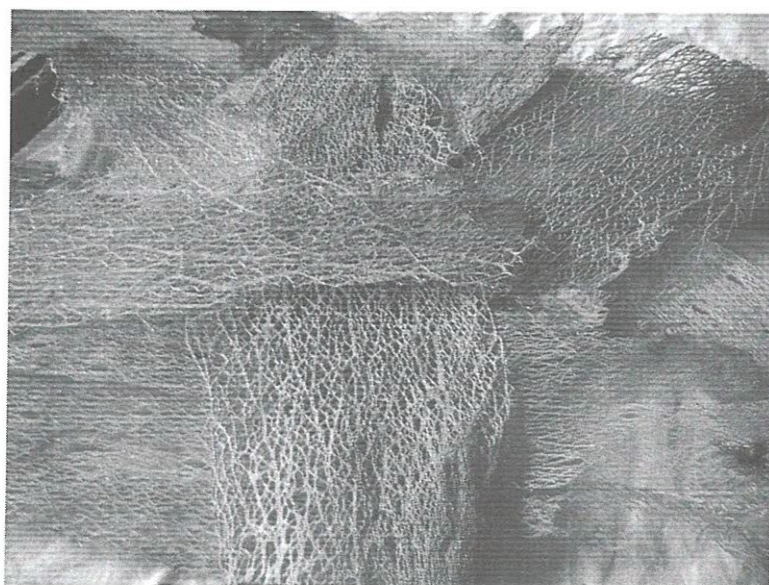
Figure II.4. Fibres de cactus obtenue.
