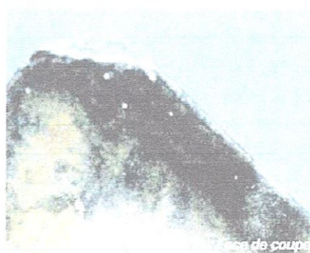
Figure I-22 Rupture de la plaquette [TRA06].
