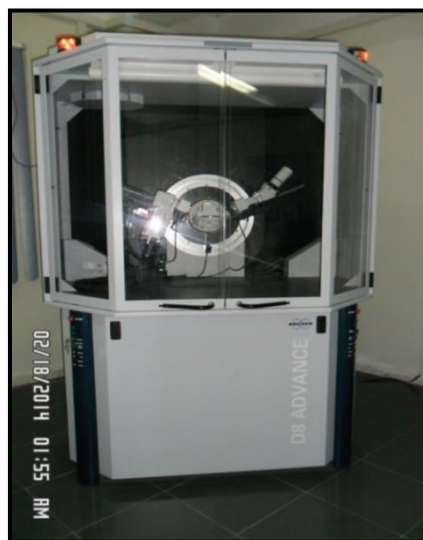
Figure III.5: Diffractomètre de marque Bruker de type D8 Advance
