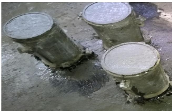
Figure II.4: Epreuves cylindriques 160x320 mm.
