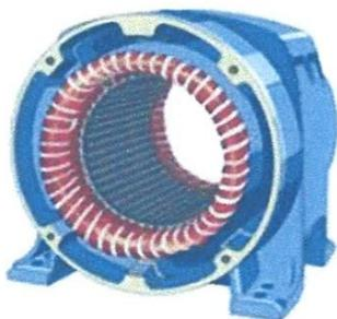
Figure (I-1): Stator
