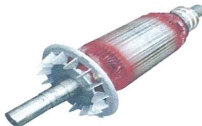
Figure (I-2): Rotor bobinée
