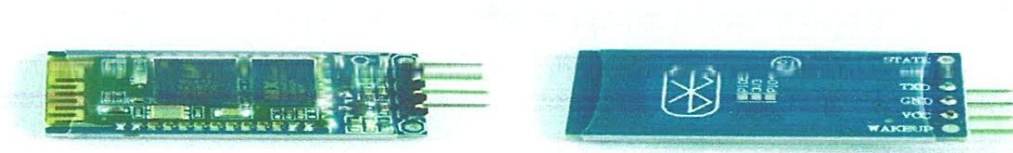
Figure 2.2: Le module Bluetooth " HC-06"
