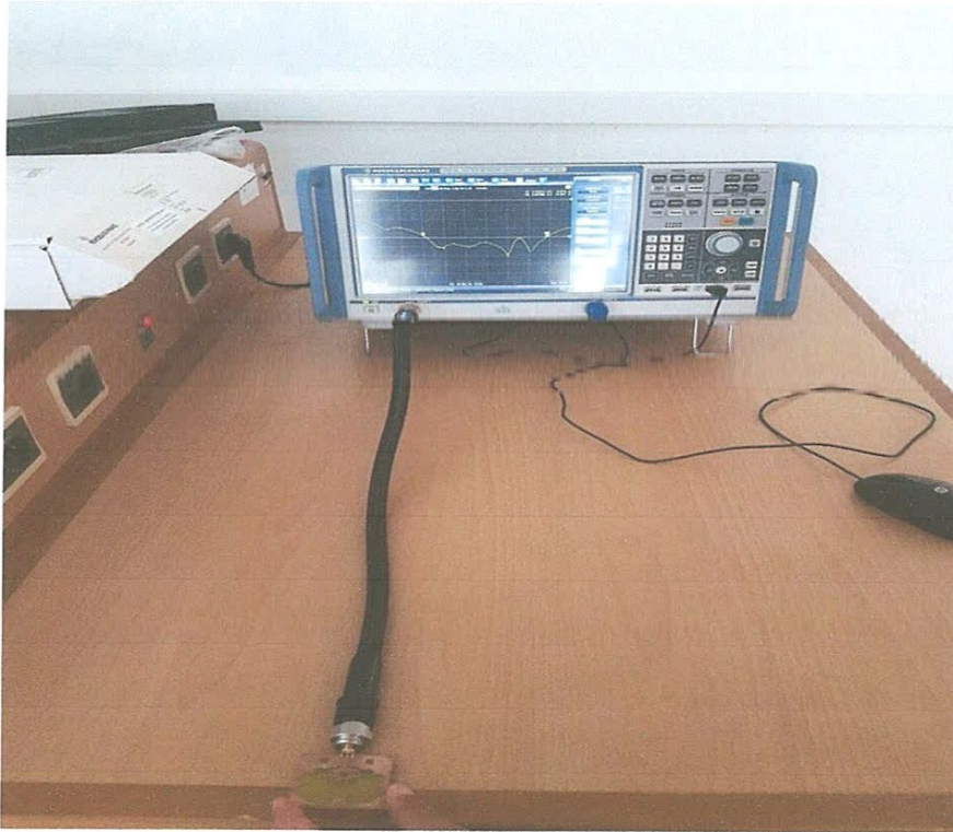
Figure III.15 ZNB 20-VECTOR NETWORK ANALYZER-100 kHz-20GHz
