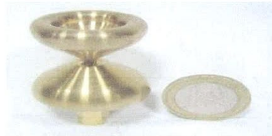
Figure II.9: Photo d'une antenne biconique [II.8]
