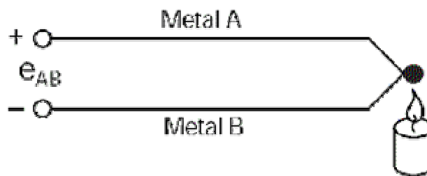
Figure 3.2 e_{AB} tension Seebeck [11].
