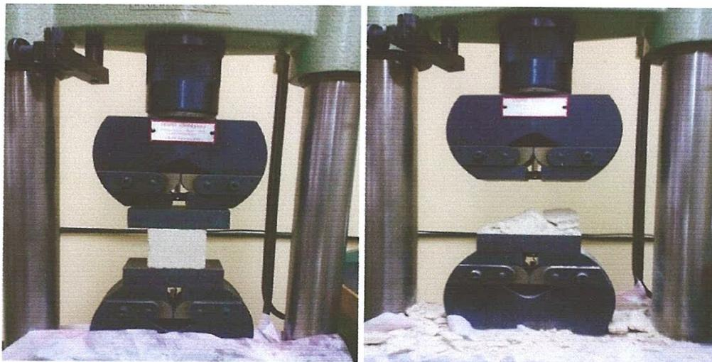
Figure 29: Essai de compression
