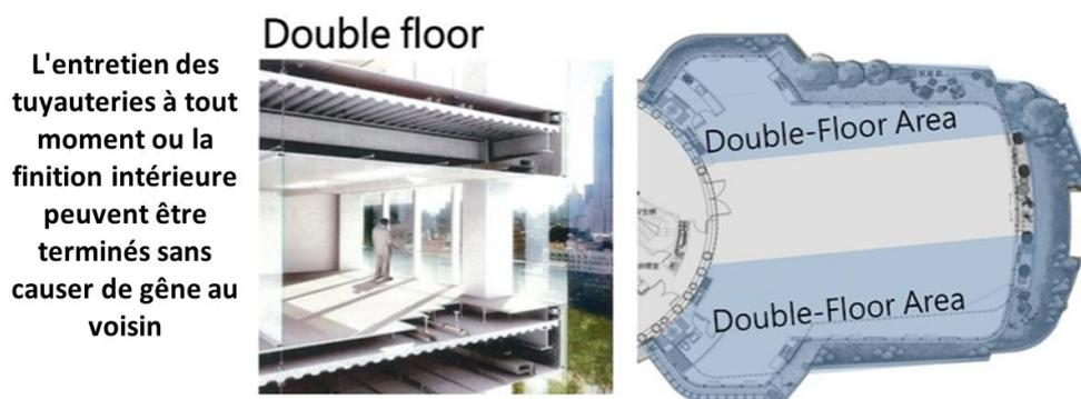
**Figure 125 :** système de double plancher. (Source : <https://www.flickr.com/photos/eager/15365389816/in/photostream/lightbox/>)
