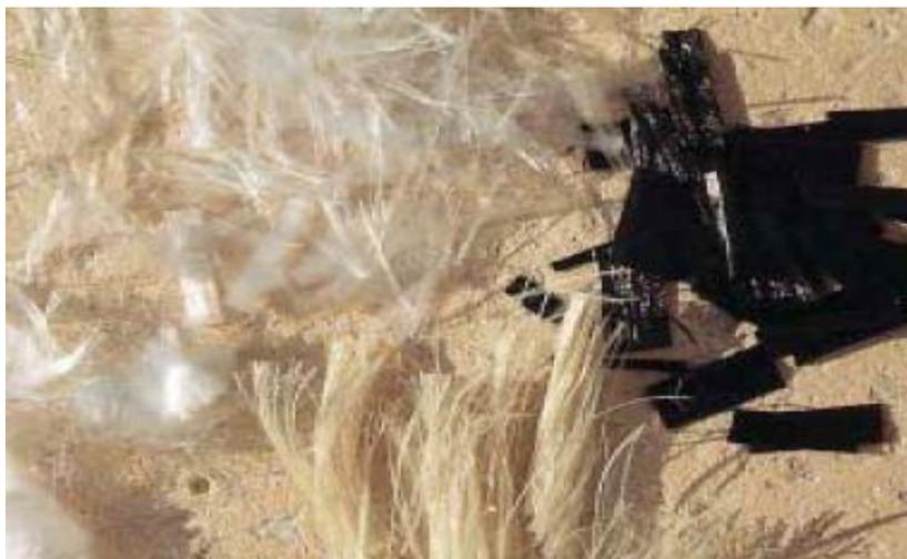
**Figure I.6.** Photo des fibres polypropylène (FPP), [Yagoub. M, 2009].
