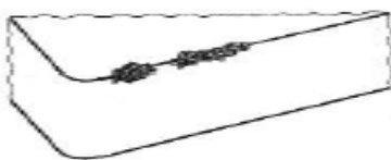
Figure I.23: Rupture de la plaquette [20]
