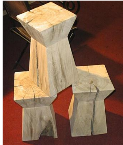
Figure 1-6: fissure de retrait
