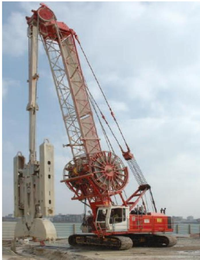
**Figure 1.21** Benne hydraulique KS2
