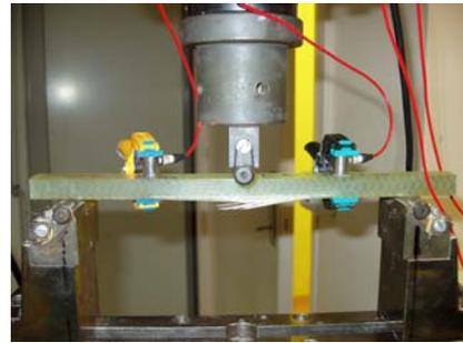
Fig. 5 Set-up for the acoustic events
