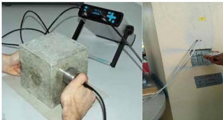
Fig 3.14. Non-Destructive Testing Methods for Concrete Evaluation [44].
