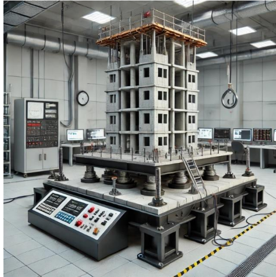
Fig 2.20. Shake Table Testing Setup [8].
