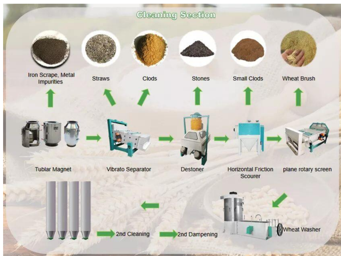
Figure 3: Cleaning section of wheat (source: https://www.chinagrainmachine.com ).
