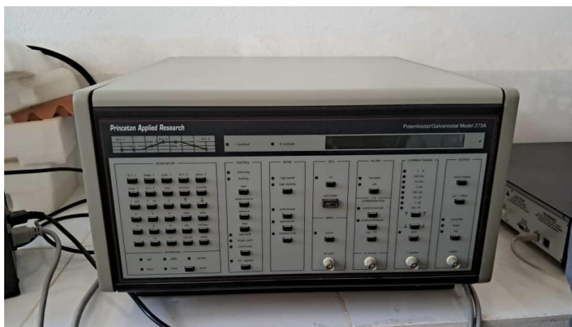
Figure III.19. Experimental setup used to characterize the sensitivity of the developed sensors developed by SWV.
