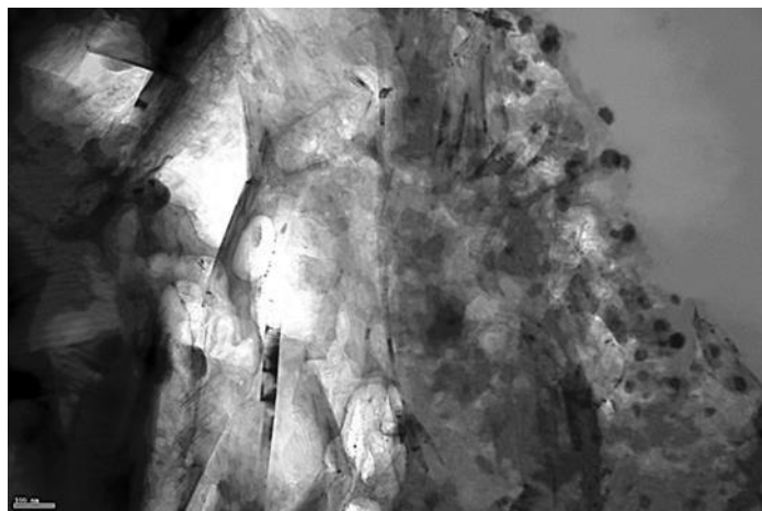
Figure IV.4. TEM image of RuNPs deposited onto ASPE.
