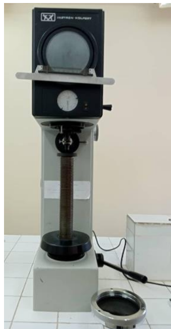
Figure 3: Experimental setup for microhardness testing.
