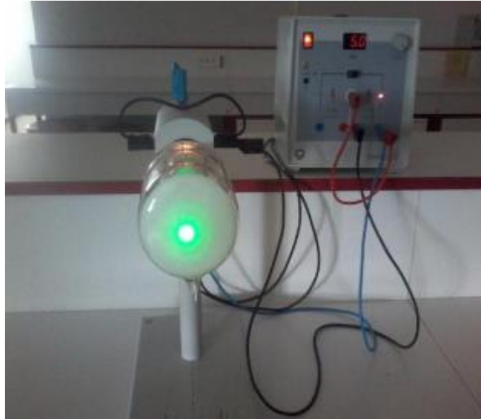
Figure 4: Experimental setup for electron diffraction.
