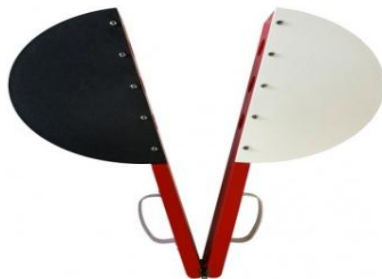
Figure 3-20: Starter Clapper Used to generate the Impulsive Noise. Source: (author).
