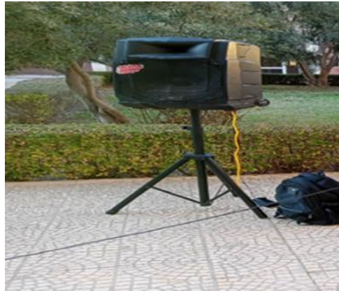
Figure 3-19: Directional speaker used for generating white noise. Source: (author).
