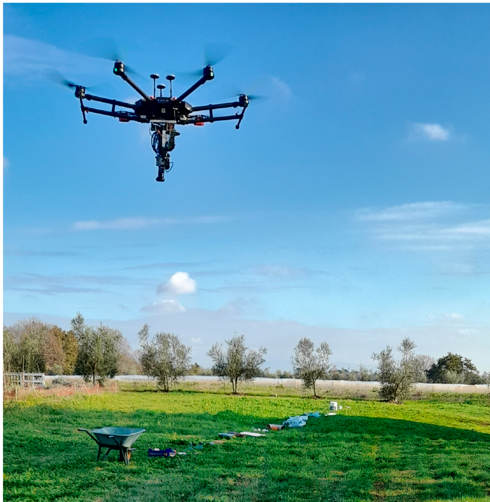
FIGURE 3.4 – Aerial hyperspectral-survey setup showing the SWIR camera mounted on the UAV, white reference tiles, and arranged plastic samples [5].
