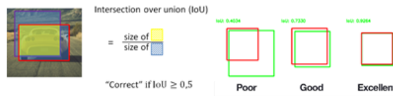
FIGURE 2.3: Intersection over union and example of IoU
