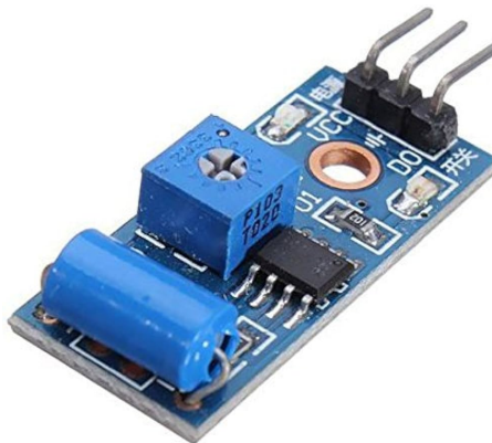
Figure 2.4 – SW-420 Vibration Sensor Module [W38]
