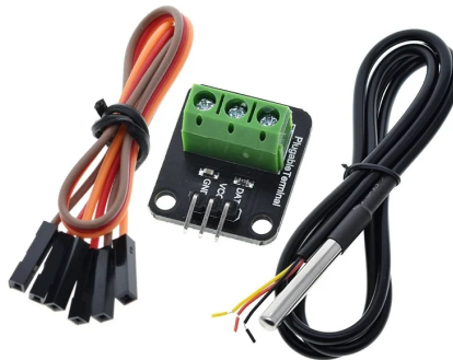
Figure 2.6 – Temperature Sensor DS18B20 [W40]
