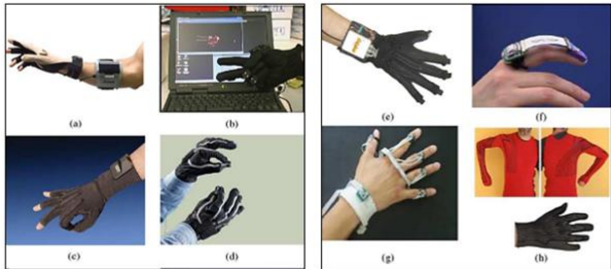
Figure 1-13 Examples of Glove systems: (a) CyberGlove, (b) Humanglove, (c) Pinch Glove (Image courtesy of Fakespace Systems), (d) Didjiglove, (e) Fingernail Sensor [Ghu14], (f) AcceleGlove [Her02], (g) Upper limb garment prototype [Par06], and (h) Sensing glove [LS T05].
