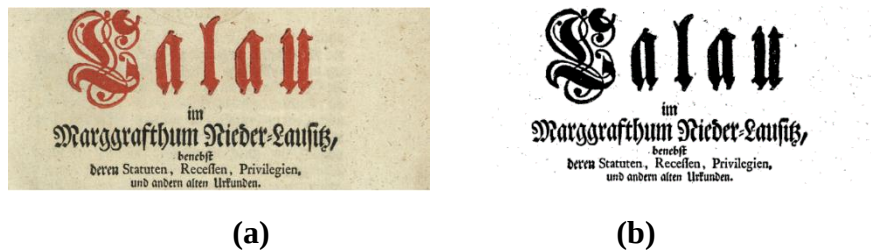
Figure 1.1. Example of binarization, (a) original document, (b) its binary representation.
