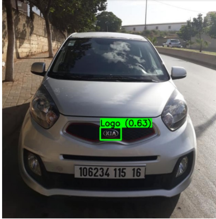
Figure 3.32: Sample Results of Vehicle Logo Detection using YOLOv8
