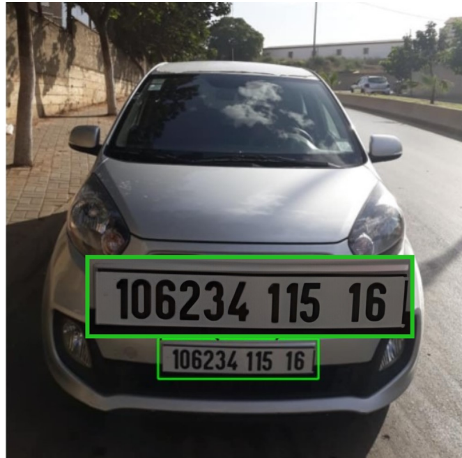
Figure 3.25: License Plate Extraction Result Using YOLOv8
