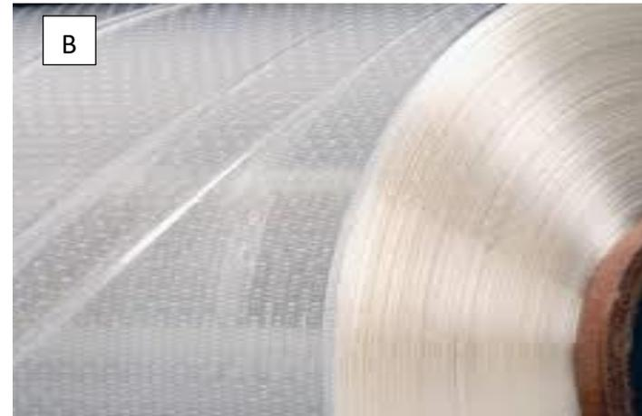
**Figure II.2 :** (A) tissu d'arrachage, (B) tissu perforé
