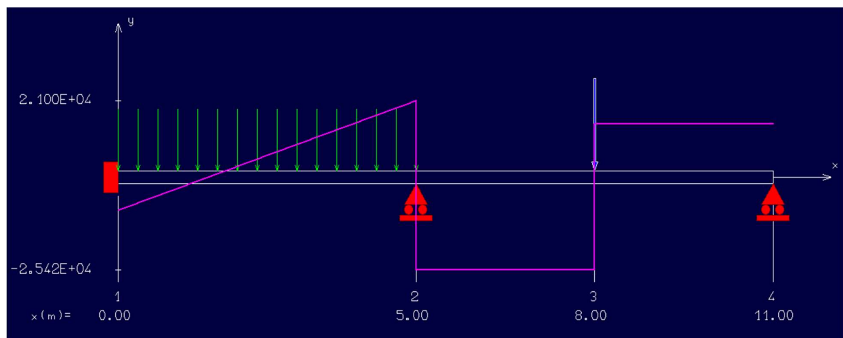
Fig. 17: Distribution of bending moments (kNm) along the entire length of the continuous beam
