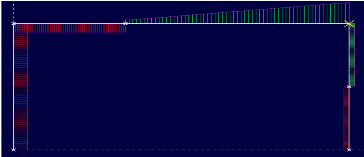
Fig. 10: Shear force distribution along the frame
