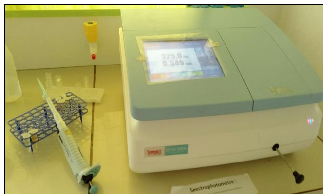
Figure 12: The spectrophotometer for measuring the UV-vis absorption spectra of the ethanolic extract of propolis (EEP).
