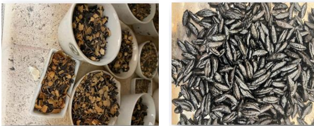
Figure 6: Eggshells and date seeds biomass after pyrolysis
