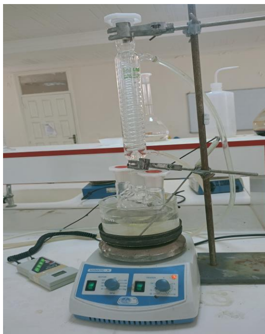
Figure II.6. Montage a reflux.
