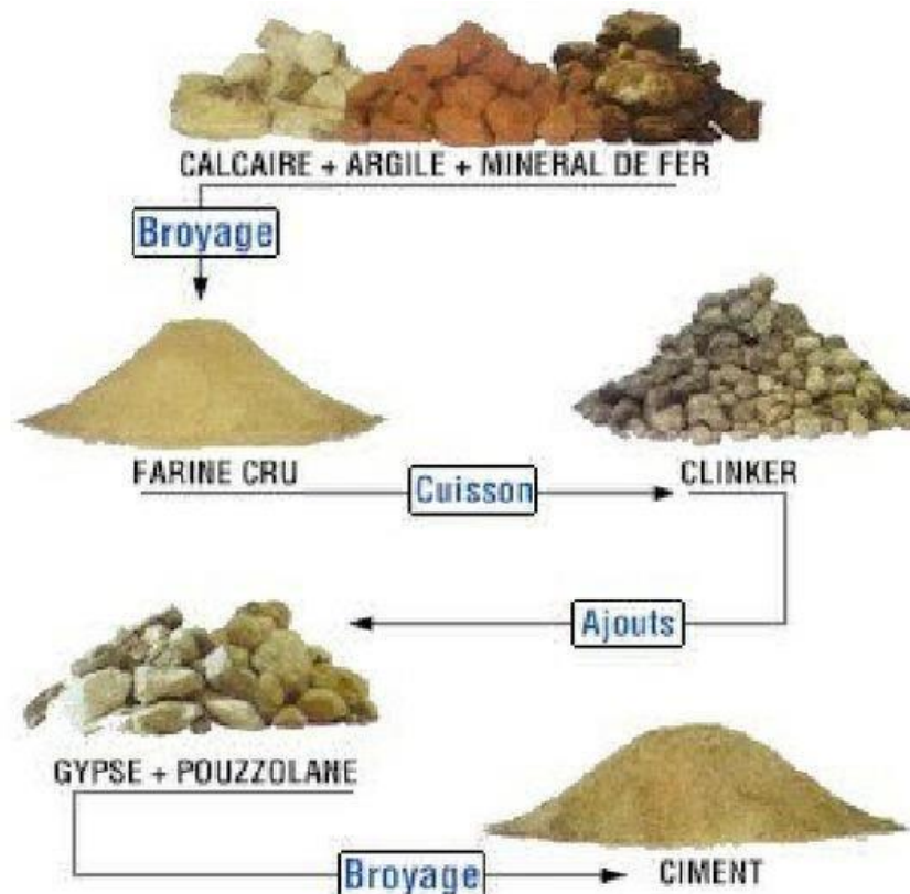
Figure II.13. Processus de fabrication de ciment.
