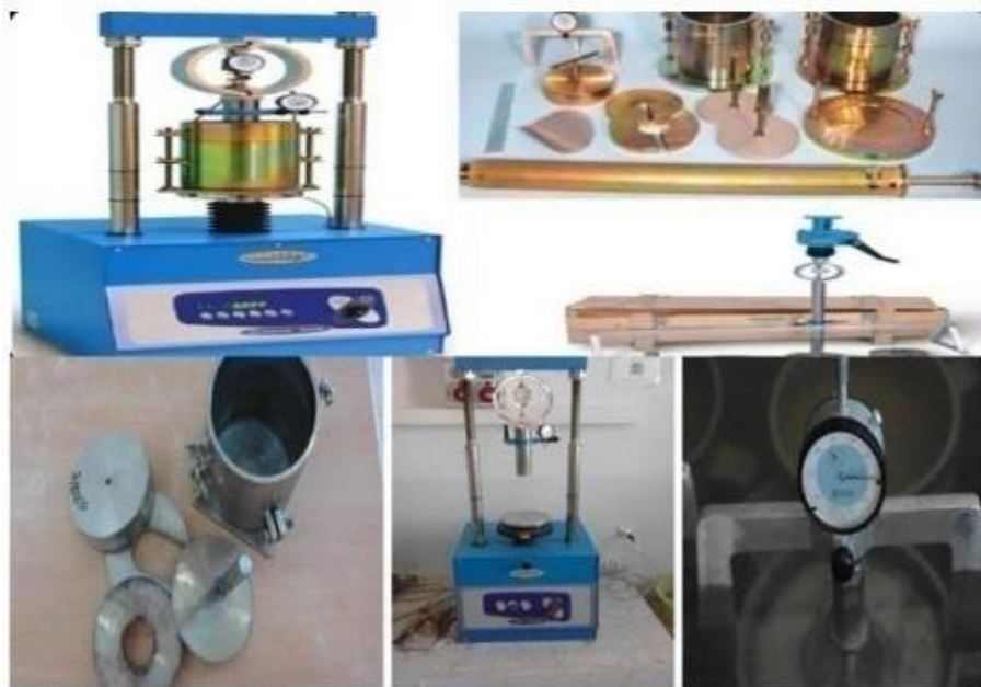
Figure III.23. L'essai CBR (California Bearing Ratio).
