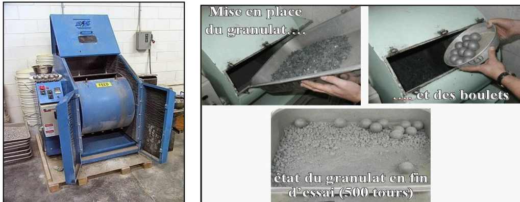
Figure III.10. Essai Los Angeles
