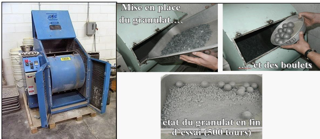
Figure III.6 : Essai Los Angeles.
