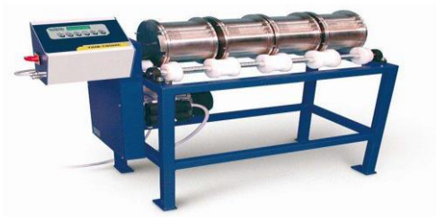
Figure III.8 : Machine Micro-Deval le MDE
