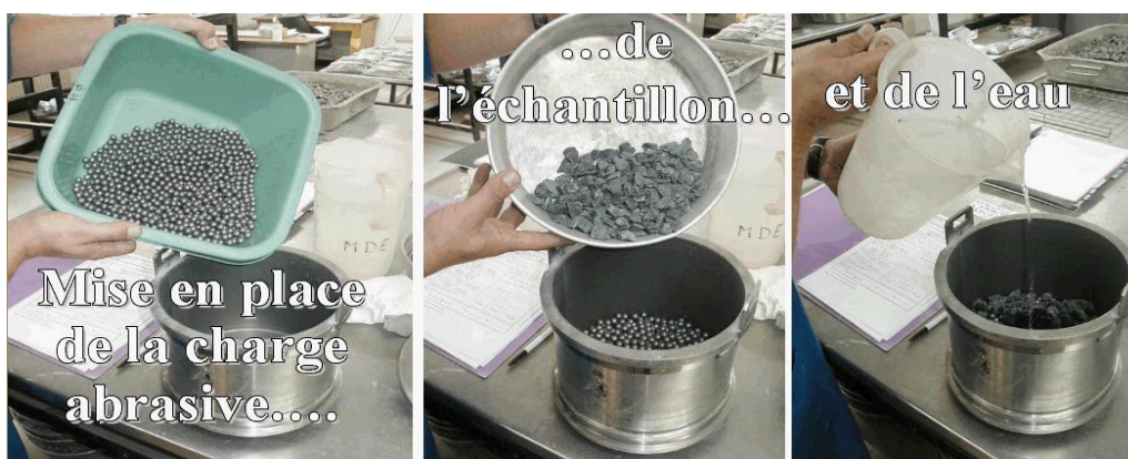
Figure III.7 : Essai Micro Deval.
