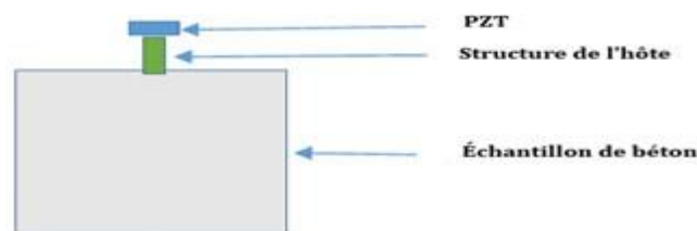
Figure II.3.7: Illustration of indirect interaction of PZT to monitor concrete characteristics [WASSEM et al., 2022].
