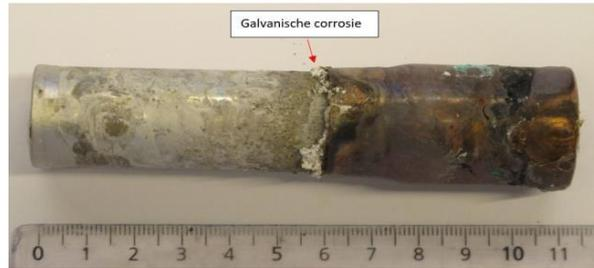
**Figure 2.22 :** Corrosion galvanique [43].
