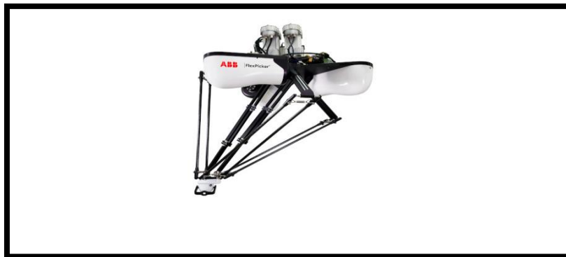
Figure I.5 : FlexPicker, robot delta ultrarapide
