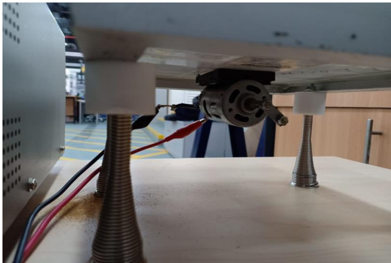
Figure III.5. Vibration tech for self-cleaning solar panels [56]
