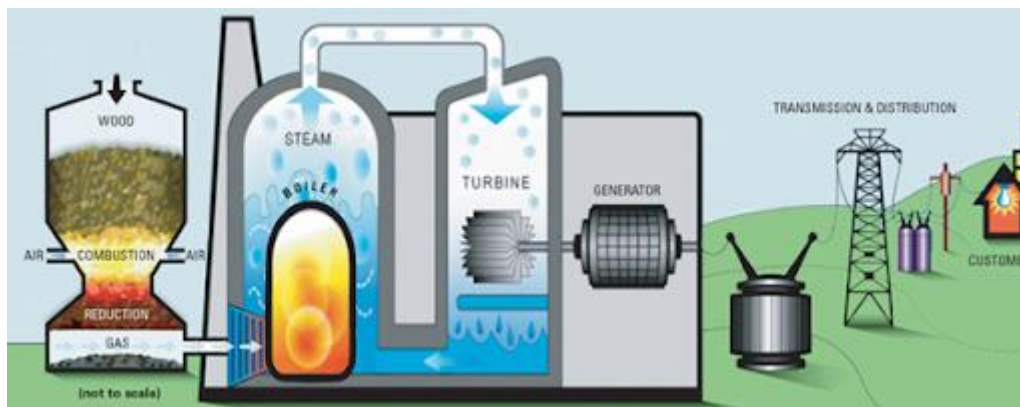
Figure I.13. Biomass gasification power generation technology [31]
