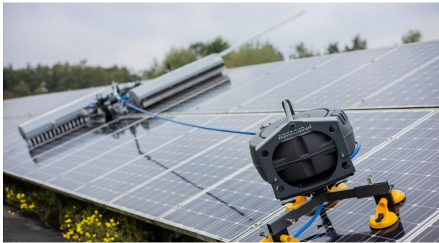
Figure III.4. Photovoltaic cleaning robot [55]
