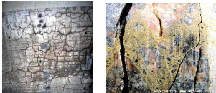
Fig 5.8: Degradation of concrete due to the alkali-silica reaction.
