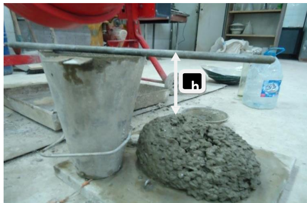
Figure II.12: Abrams cone slump test (University of GUELMA).
