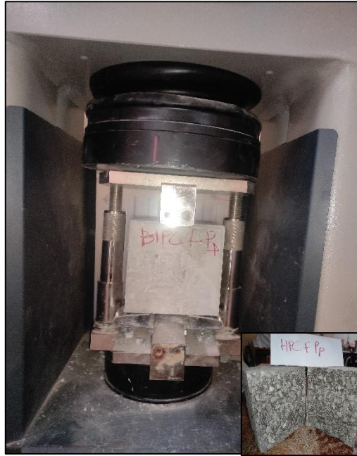
Figure III.3: Tensile strength test
