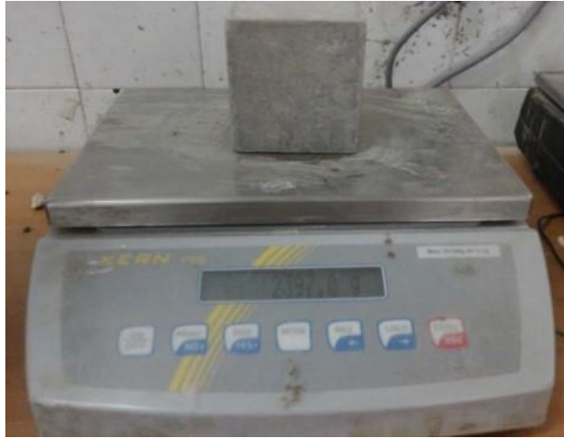
Figure III.1: Measurement of mass loss (LGCH, University of GUELMA)
