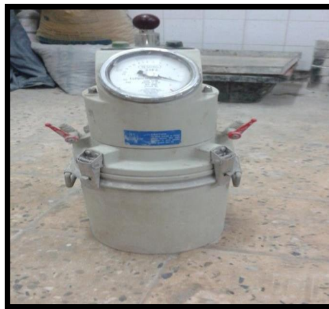
Figure II.13: Concrete air meter (University of GUELMA).
