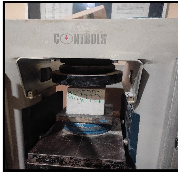
Figure III.2: Compression test (LGCH, University of Guelma).
