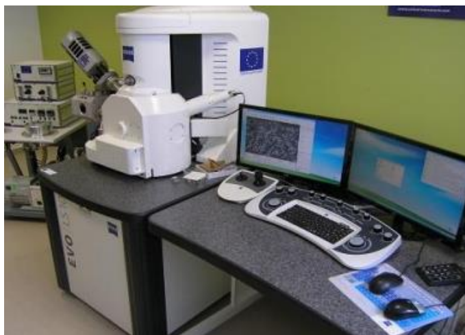
Figure III.8. Field emission scanning electron microscope coupled with energy dispersive X–ray spectroscopy ZEISS EVO LS10.
