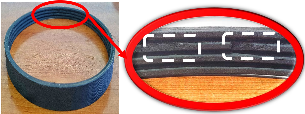
Figure 3.19. Defects identified on the V-ribbed belt.
