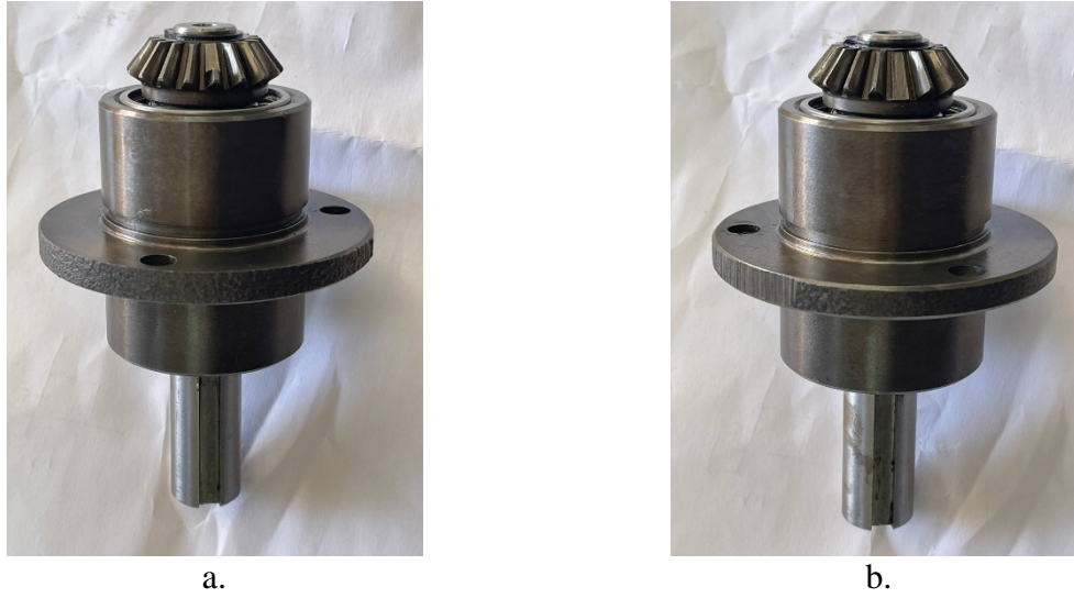
Figure 2.4. Defective gear: a. half tooth extracted, b. tooth extracted completely.
