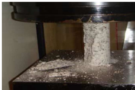
Figure III.6 Uniaxial compression test on a granite
