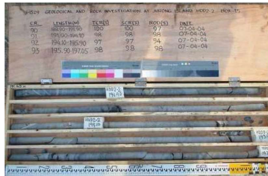
Figure I.24 Example of measuring RQD from core logging
