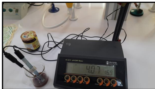
Figure 12: The measurement of the hydrogen potential by pHmeter ( personal plug ).
