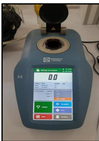
Figure 14: The refractometer for Brix measurement ( personal plug ).
