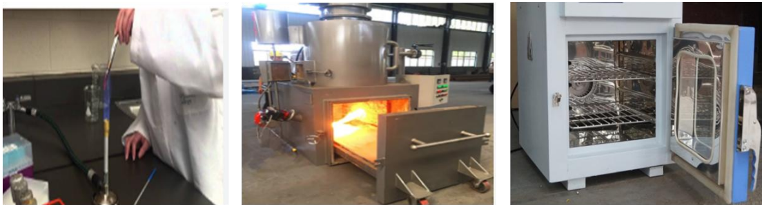
Figure 9. Dry heat sterilization methods: flaming, incineration and hot air oven.
