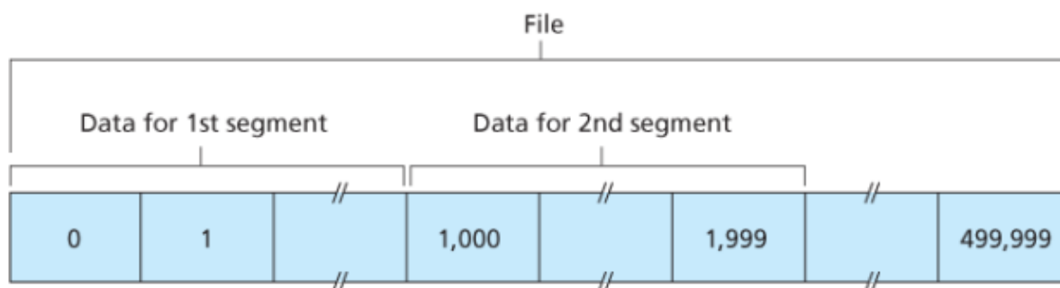
Figure 1.11: Dividing file data into TCP segments [8]
