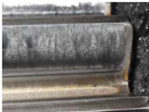
Figure III.24: Grippage à chaud [25]
