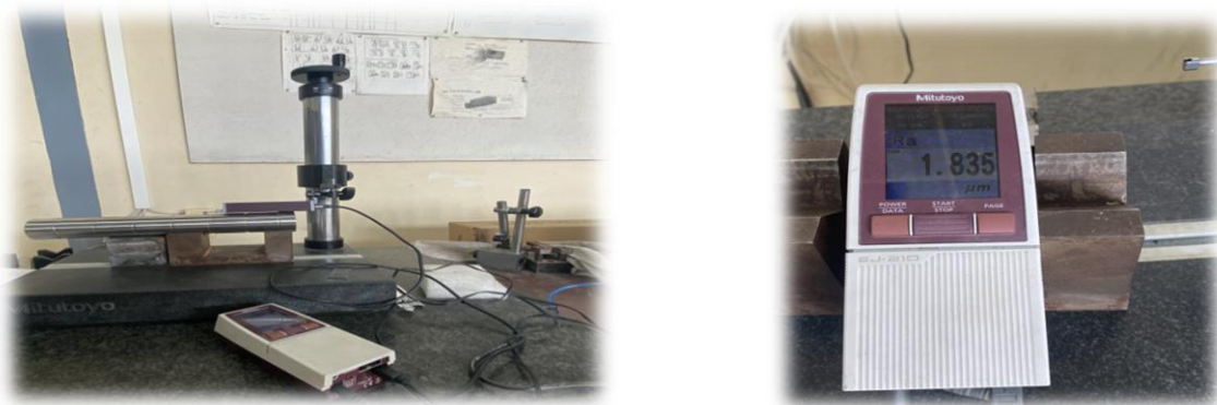
Figure II.5: Rugosimètre Mitutoyo SJ-210 (2D).
