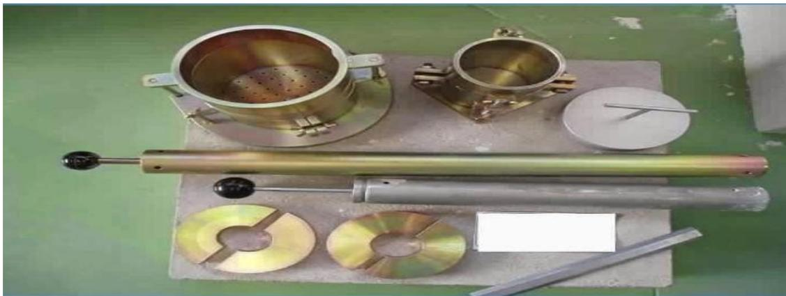
Figure III.6: l'essai Proctor
